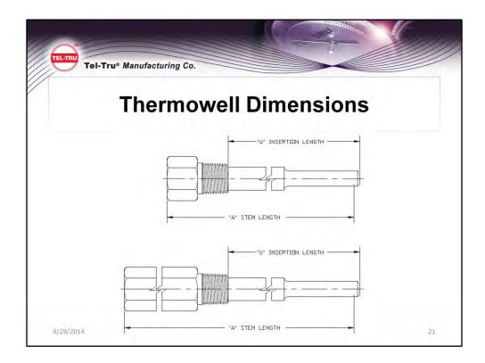
These illustrations show a well with and without a lagging extension. A lagging extension is common when there is insulation or you want the head of your instrument further away from the process.
