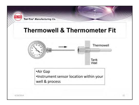
Temperature transfer from the thermowell to thermometer can be slowed by the air gap between them, and delay the thermometer reading response time.
