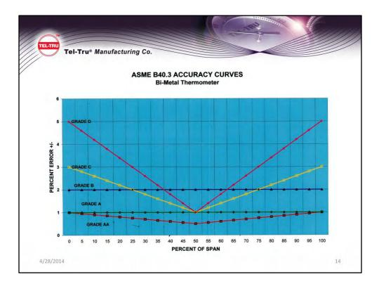
The accuracy curves for bimetal thermometers is shown in this chart. The Grade A = +/- 1% full span and is common in the USA. The grade AA is achievable by manufacturers that make their own bimetal coils.
