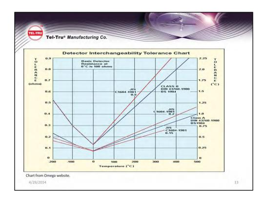
RTD sensors are specified according to their resistance in ohms at zero degrees Celsius. A PT100 element measures 100 ohms at 0° C. The electrical resistance measured in ohms increases as temperature increases. Prompting a repeatable resistance versus temperature relationship.
