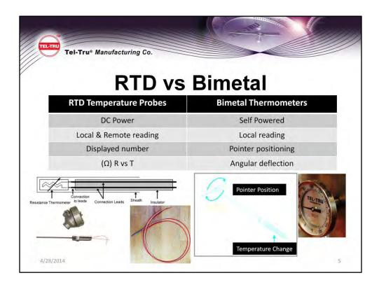
**RTD temperature probes** are widely used because of their accuracy and repeatability. RTD's are typically made with platinum wire elements, an electrical resistance source. An electronic circuit is used to convert the resistance value into a temperature reading. The change in electrical resistance is indicated as a temperature reading on a digital display or meter.
