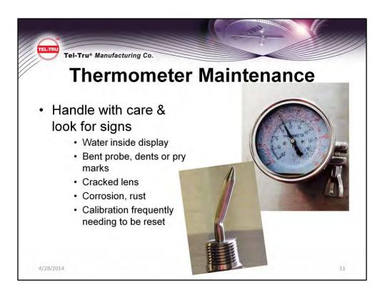
Thermometers are calibrated instruments – that need to be handled with care. Look for visible signs of a problem such as water inside the case.
