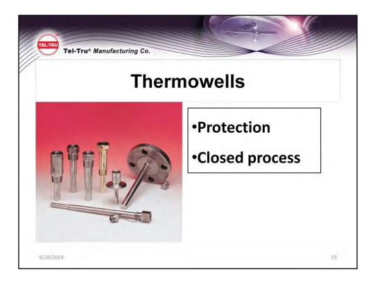
Installing a thermowell will help protect your thermometer and allow you to remove the thermometer without shutting down your process or draining your tank. A Thermowell is a drilled out piece of solid metal barstock that is machined with a process connection and shank suitable to the process conditions and fit with your instrument.
